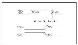
Figure 1. Modulus Control Timing Diagram
